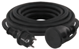
P01805 19 21 010 504 1/-/-/20 ↔ 5 m Black cable 230 V~/16 A max. / \Sigma 3 680 W max. / H07RN-F3G 1.5 mm 2 / IP44 / Rubber + neoprene 8 592920 064566
