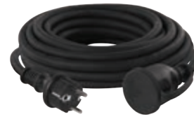
P01810 19 21 031 000 1/-/-/6 ↔ 10 m Black cable 230 V~/16 A max. / \Sigma 3 680 W max. / H07RN-F3G 1.5 mm 2 / IP44 / Rubber + neoprene 8 592920 011058
