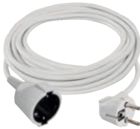
P0125R 19 21 010 503 1/5/-/20 ↔ 5 m White cable 250 V~/16 A max. / \Sigma 3 680 W max. / H05VV-F3G 1.5 mm 2 / PVC 8 592920 064481
